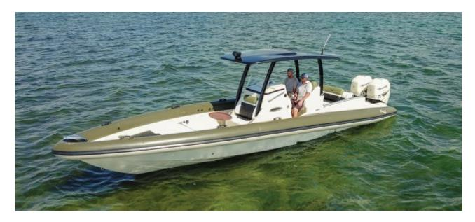
The **Airship 340** replaces the builder's 330 and adds high-quality features. The remodeled transom includes an incorporated engine setback, a step for boarding and extended swim platform for watersports. Construction features remain consistent and utilize varying density foam cores and vinylester resins to form a lightweight, yet a strong vessel.
