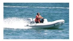
The advantages of this new design include better weight distribution by moving the weight of the gas tank forward and clearing the deck area of the clutter. Powered by a 20-hp motor, she runs to a top speed of 25 knots. All Achilles boats are manufactured with CSM fabric using a four-layer seam construction for durability.
